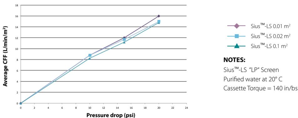
Graph 1: Pressure drop vs. cross-flow flux - Sius™-LS "LP" screen
