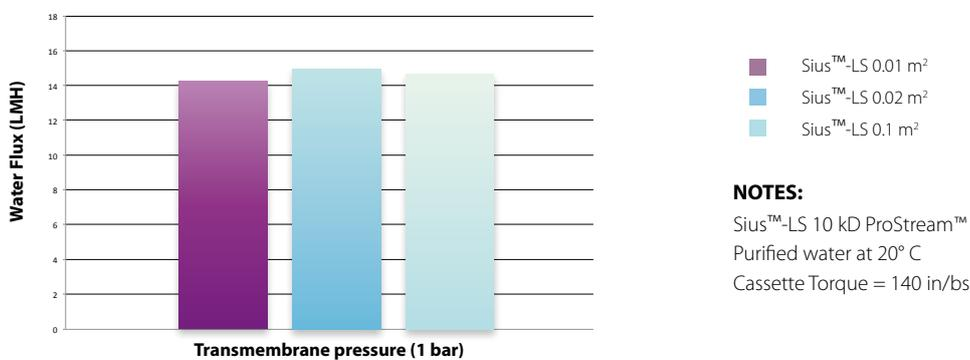
Graph 2: Transmembrane pressure vs. water flux - Sius™-LS 10 kD
